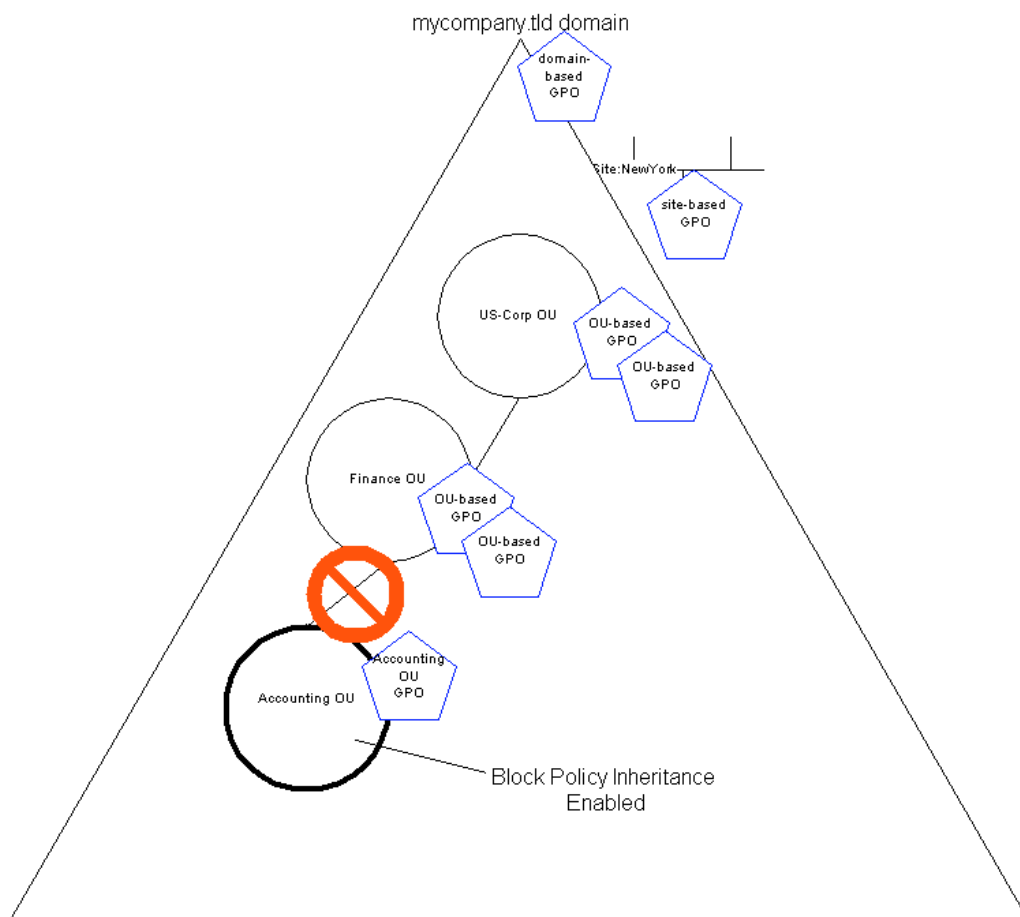
Figure 3.6: Blocking policy inheritance in an AD domain.
