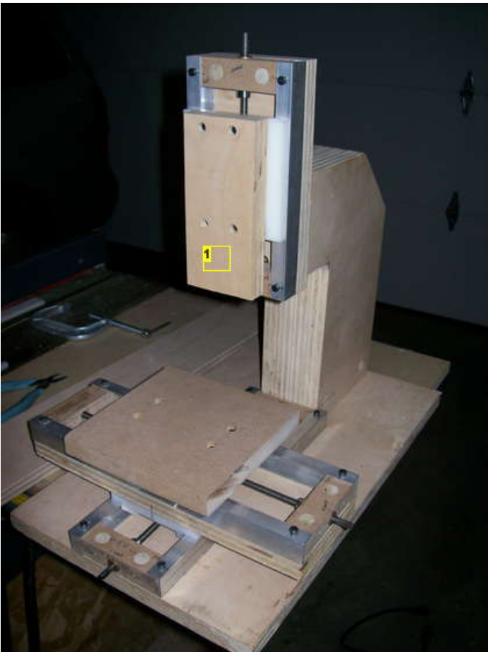
Image Notes 1. motor base plate- it sits flush with the top of the Z axis slide
