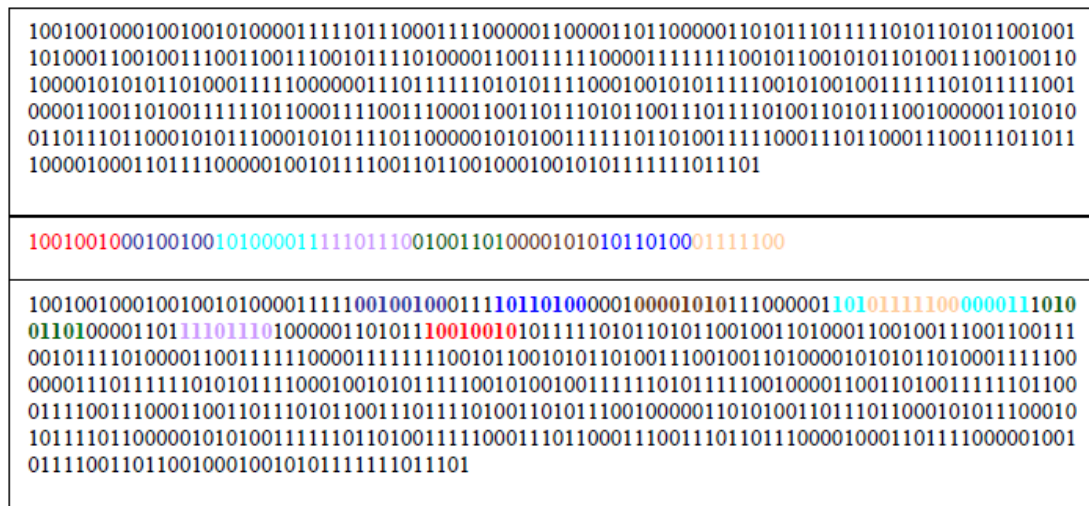
Figure 2 : Insert every 8 bit from the key to the specific index in the data.
